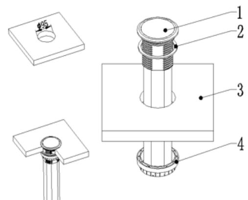
1: Top, 2: Silicon Pad / Metal Washer, 3: Bench-top, 4: Mounting Ring
